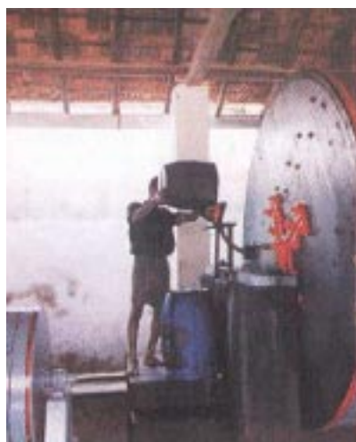
Poor arrangements and practices in dosing acids (Source: UNIDO)
