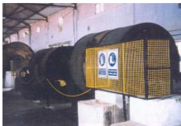
Guarding access to a drum in a small-scale tannery (Source: UNIDO)
