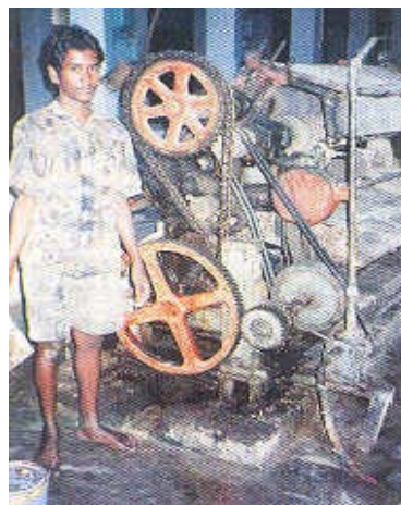
Poorly guarded fleshing machine (Source: UNIDO)
